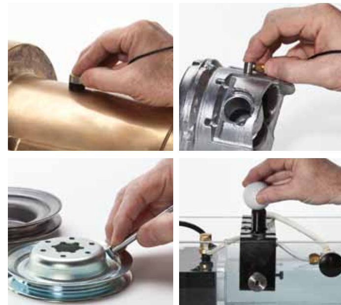
Ultrasonic thickness measurements are accurate, reliable, and repeatable. Instant readings can be achieved from one side of a material, making it unnecessary to cut up or destroy the part.
